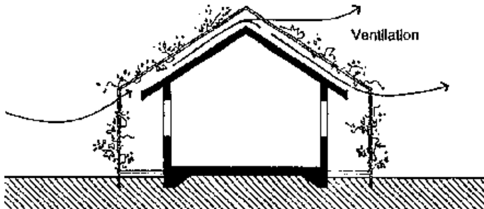
Fig 3/147 Green cover on roofs and walls
